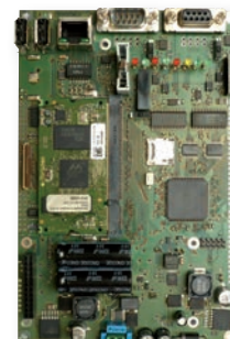
Figure 2: Chimaera Lu750 embedded system board
