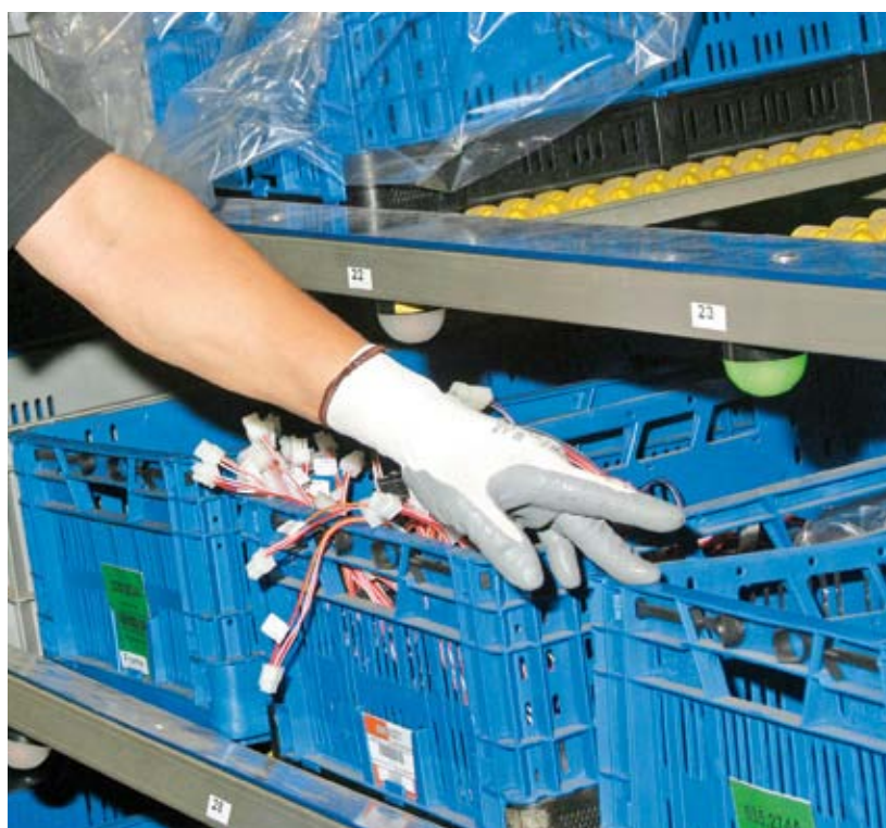
The LED lights from the pick-to-light system show the assembler from which output tray he has to pick the next component
